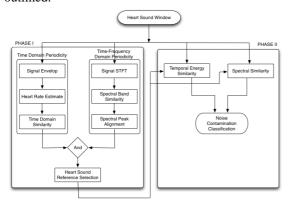
Fig. 2: Noise detection algorithm.
