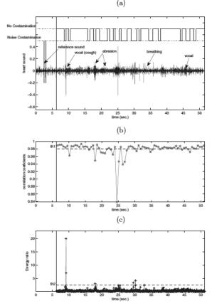
Fig. 4: (a) Noise contamination detection results. (b) Spectral correlation feature. (c) Temporal energy feature.
