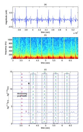
Fig. 3: a) Heart sound from mechanical valve. b) Spectrogram. c) Auto-correlation functions of the time-frequency bands.
