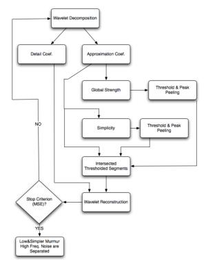
Fig. 7: Wavelet-Simplicity Filter segmentation algorithm.
